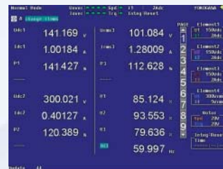
Measure the DC voltage, DC current, and power conversion efficiency
